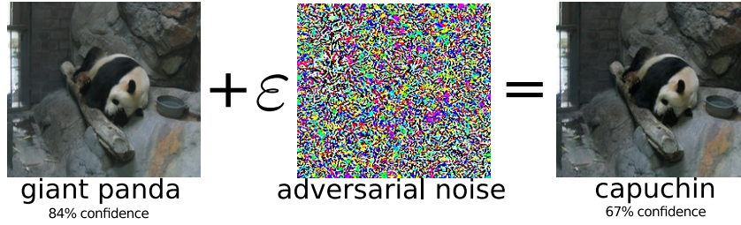
Figure 1.7 – A clean image of a panda from Imagenet dataset [53] receives adversarial noise. The obtained adversarial image still looks like a panda to the human eye, but will make the model changes its prediction to a relatively confident ‘capuchin’ label.
